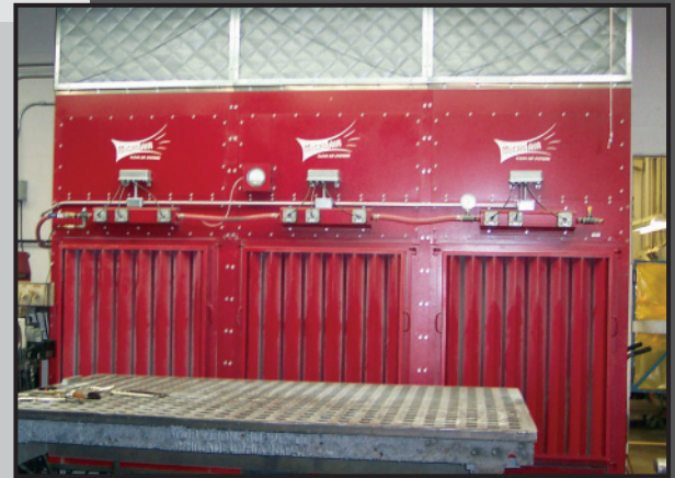
3-Module Clean Air Booth in Welding Operation
